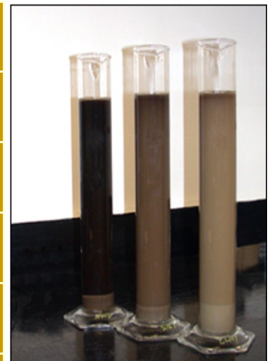
Showing the separation point between settled soils (L to R: sand, silt, and clay) and water
